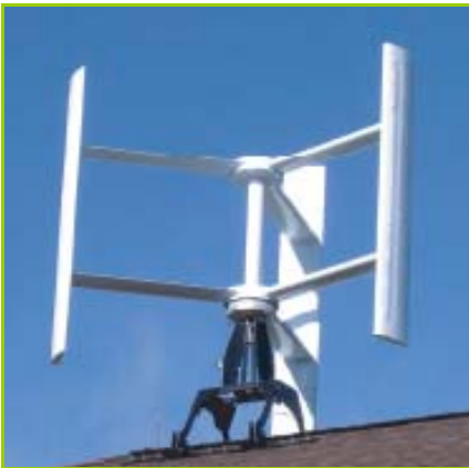
Windterra ECO-1200 turbine Rated Power Output: 1000 W
