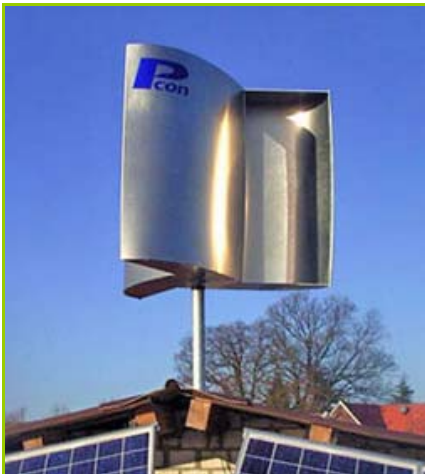
Example of a VAWT-Savonius Pcon Windkraft S3-190 Rated Power Output: 0.7kW
